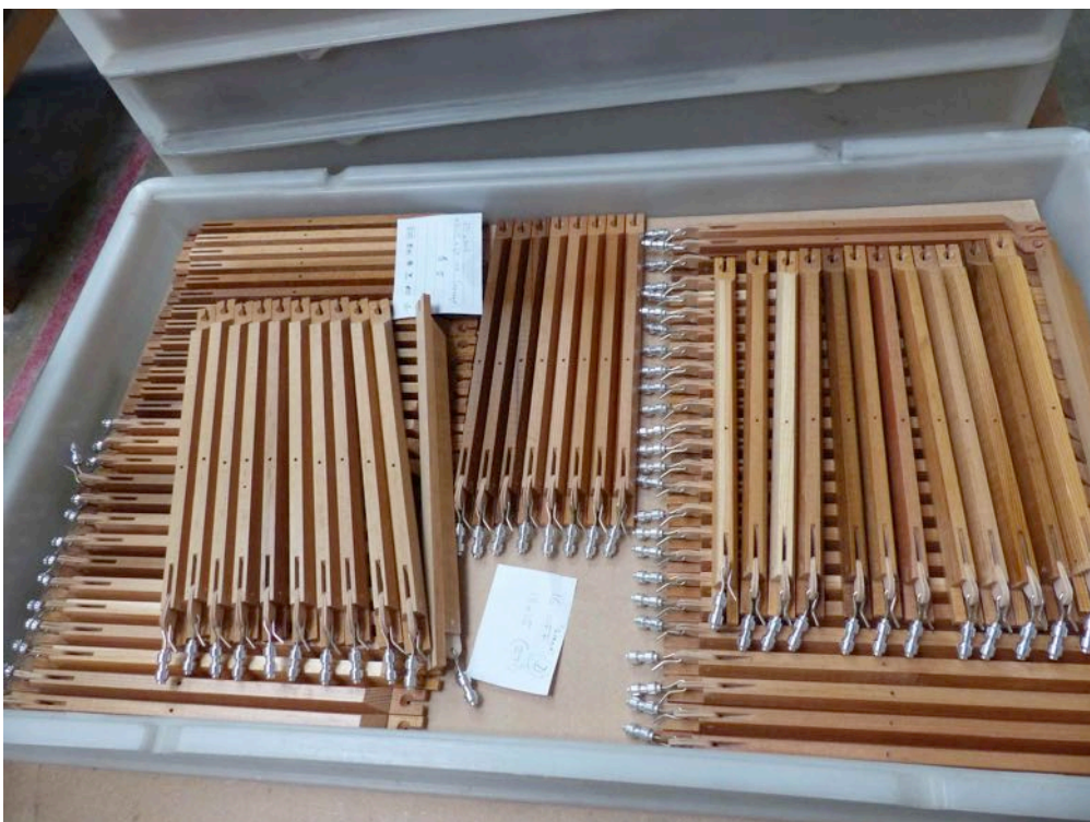
Smaller wooden parts were being made at the same time. Here are the 'pallets': the valves inside the soundboard which open to admit air to the pipes:
