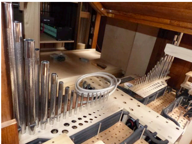
A rank of pipes in place for testing, as air runs through the organ for the first time.
