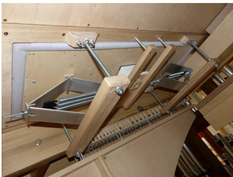
A wind pressure regulator in place beneath a soundboard, under test pressure.
